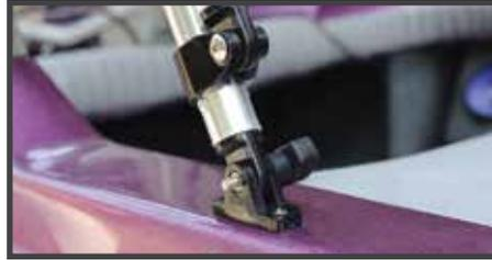
10. Install mounting hardware to the deck or side of your boat. Drill 3.2mm holes and attach the mounting hardware using the screws provided.
