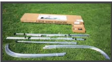
1. Open box and carefully lay out all pieces. Keep plastic on poles to reference part number until bimini is complete.
