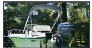
4. Zip boot sock into place to secure bimini in the collapsed position.
