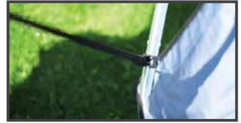
8. Attach the front support straps to the brackets in the front of the bimini.
